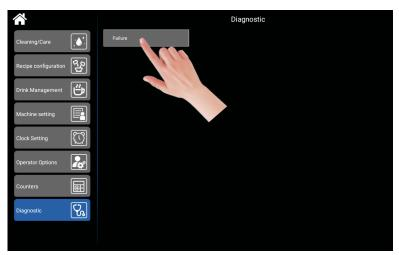
The "Failure" menu displays a list of the last errors and a list of the total errors. The user can also reset these lists or reset the machine here.
