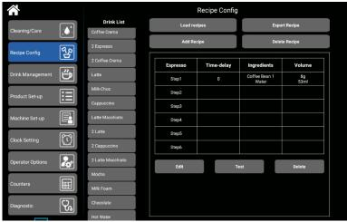
**Step 2:** In the edit recipe screen you can adjust the water volume, ingredient volume, hot milk volume or milk foam volume. Don't forget to click save and then test the drink.
