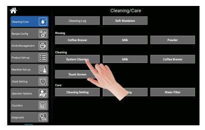
**Step 2:** In the machine interface pop-up dialog box, Press 'OK' to start the cleaning or 'Cancel' to abort.
