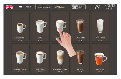
**Step 2:** Adjust the Coffee Taste Level & Cup Volume before payment "pay" mode. Click on "-" or "+" to adjust the quantity. In "free" mode, adjust the Coffee Taste Level before clicking start.
